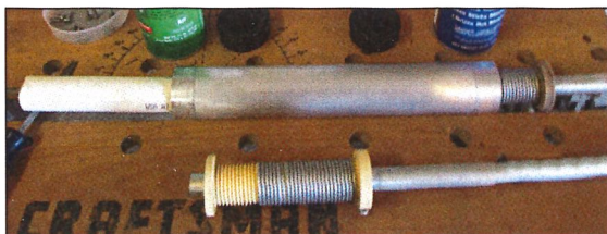
Figure 3 — Drive out a stuck trap by using PVC tubing (left) as a driver. Two black end caps can be seen above the trap.
